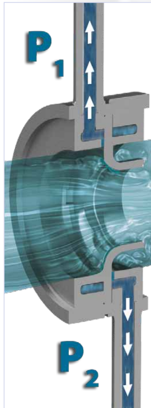
» Cross section of a chamber nozzle
